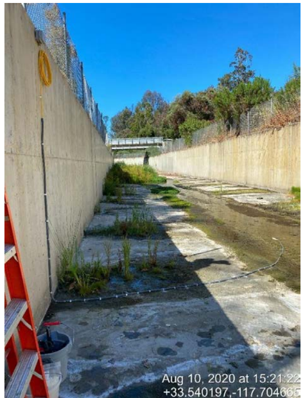
Figure 5. Example of in stream installation with smart gateway and pressure transducer.
