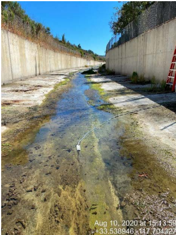
Figure 5. Example of in stream installation with smart gateway and pressure transducer.
