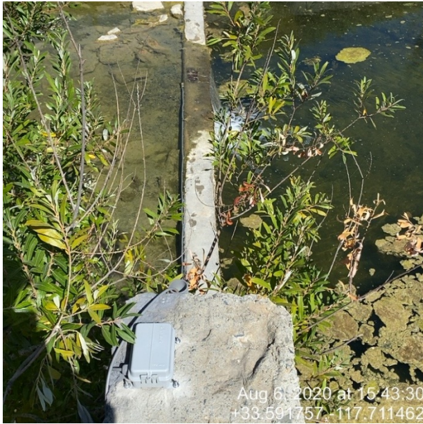
Figure 4. Example of in stream installation with smart gateway and pressure transducer.
