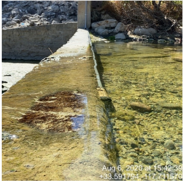
Figure 4. Example of in stream installation with smart gateway and pressure transducer.
